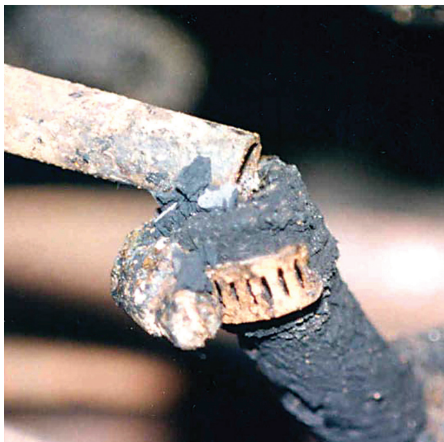
Fig. 4 — Fuel hose slipped off the metal fuel tube, resulting in a fuel related fire.
