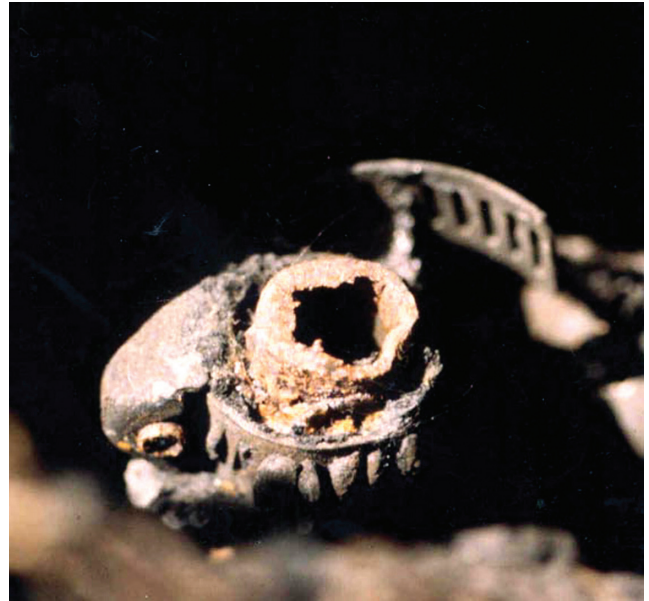
Fig. 3 — Irregular surface resulting from where a leaking area in a metal fuel tube was removed with a saw.
