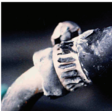
Fig. 2 — Over-torquing can cause the hose material to extrude through the grooves in the hose clamp.
